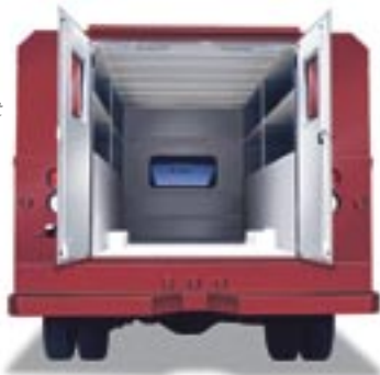
Compartment interiors painted white for enhanced illumination
